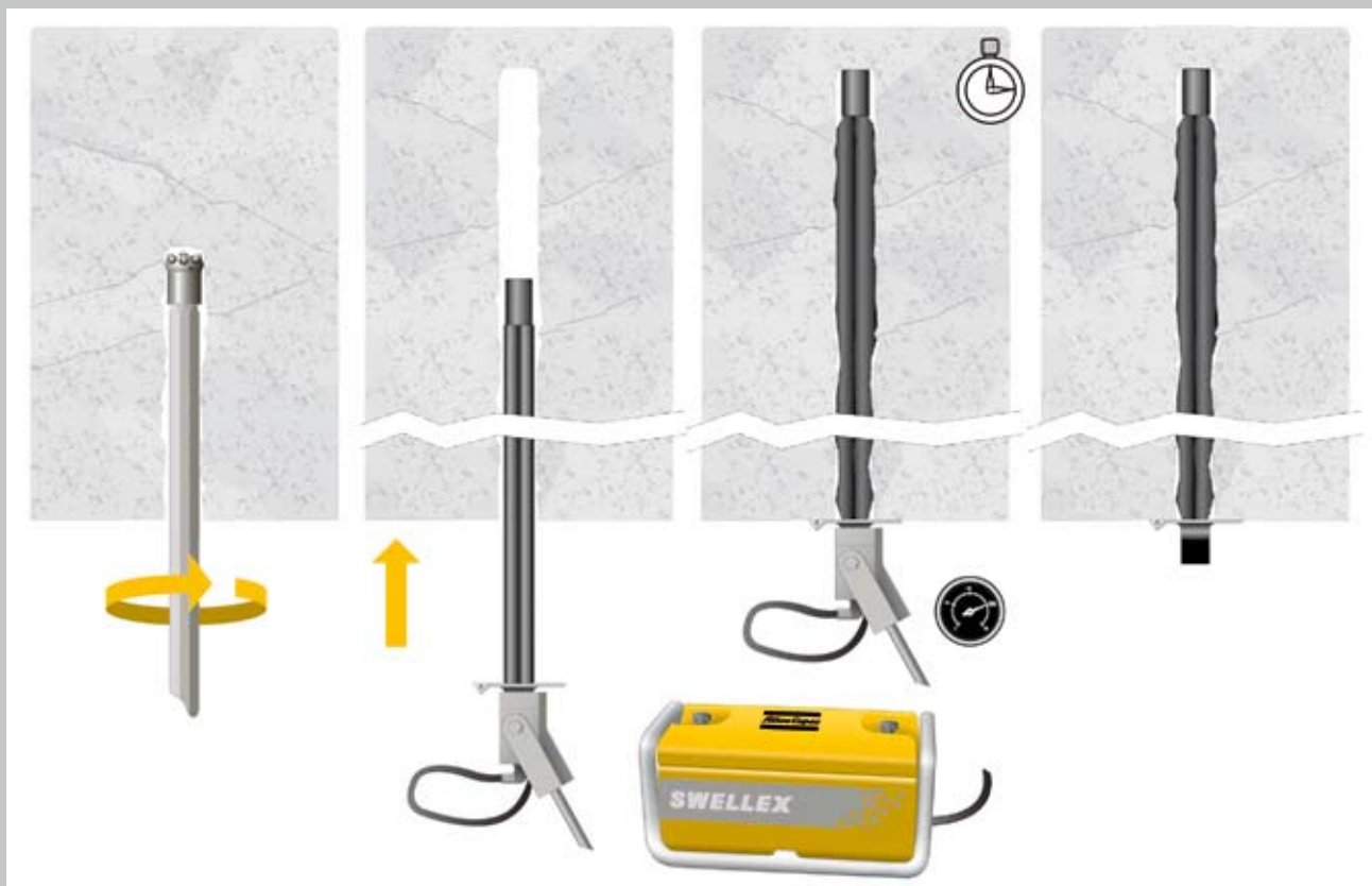
Manuelle Installation eines Swellex Ankers Manual installation of Swellex bolt
